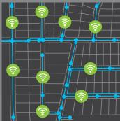
A high resolution network of iTracker sensors microdetect I&I to 3-4 manholes
