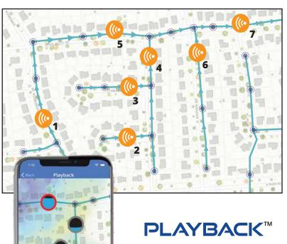
Discovering the location of I&I is as easy as viewing an animated video of the performance of your collection network using any mobile device. Easily watch the effects weather-related I&I has on your wastewater system (updated every 5 minutes). Manhole segments contributing the highest volumes of I&I are automatically highlighted by red rings.
